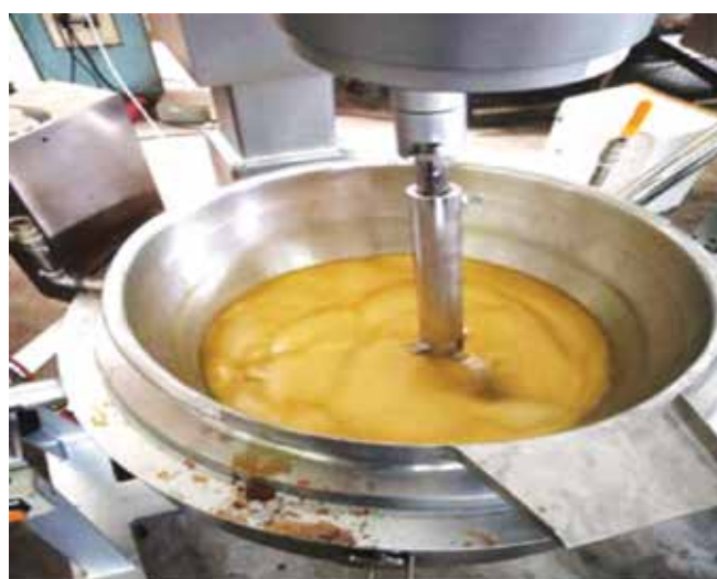
ENERGY EFFICIENT JAGGERY PROCESSING USING THERMIC FLUID KETTLE
