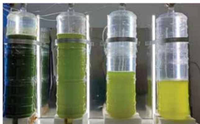
Photograph showing cultures are growing on a large scale on photo bioreactor (50 L x 4 (Cultures in each reactor are in the different stage)
