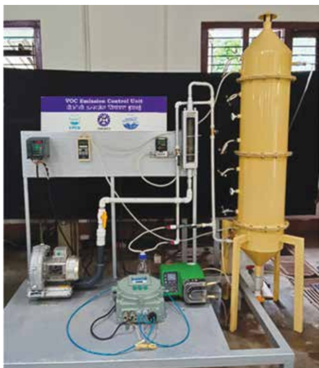
Modular VOC Emission Control Unit-Gas Bio-trickling filter
