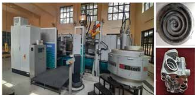
Pilot-scale squeeze casting facility (Bühler Evolution 340) at CSIR-NIIST. Scroll compressor component and engine component produced using near net shape Squeeze Casting process.
