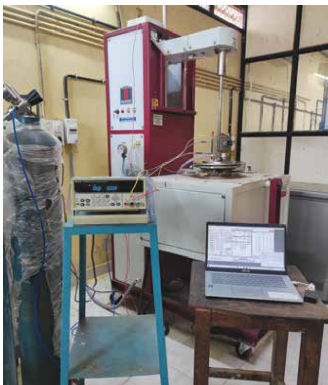
Indigenously developed high temperature molten salt electrodeposition set up for Iridium coatings
