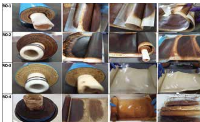
Fouled RO Membrane Filters
