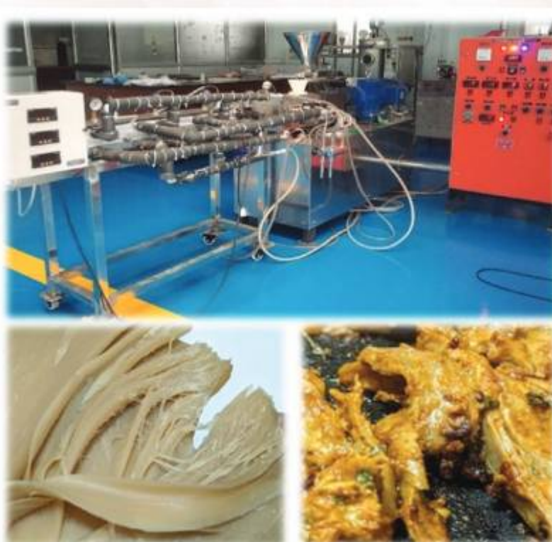
Fig. (a) Cooling die setup designed at CSIR-NIIST. (b) High moisture extrudate based on pea protein produced at CSIR-NIIST. (c) Cooked plant-based meat analogs mimicking fibrous chicken meat texture.
