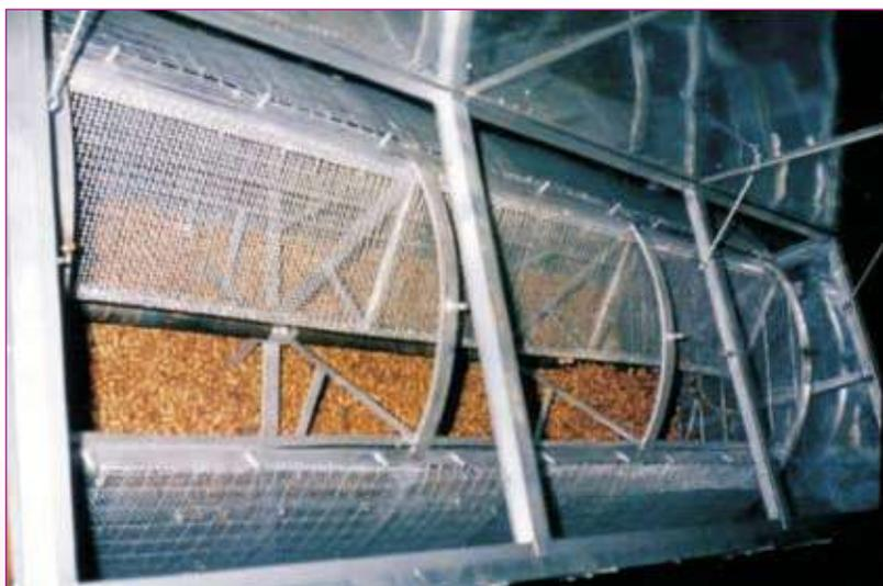
Inner cylindrical chamber of ground nut drier
