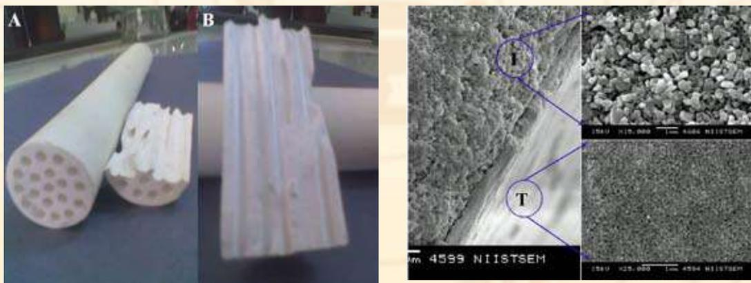
**A**-Photograph of uncoated multi channel tube, **B**- photograph of small piece of final coated tube (left). SEM image of cross section of a multilayer coating and their high resolution images with intermediate layer marked as (I) and nanotitania coated top layer (T) on right.
