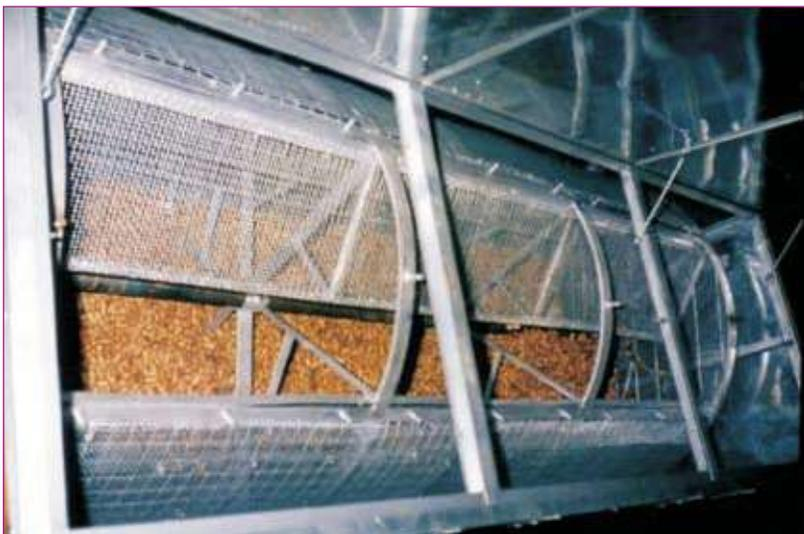
Inner cylindrical chamber of ground nut drier
